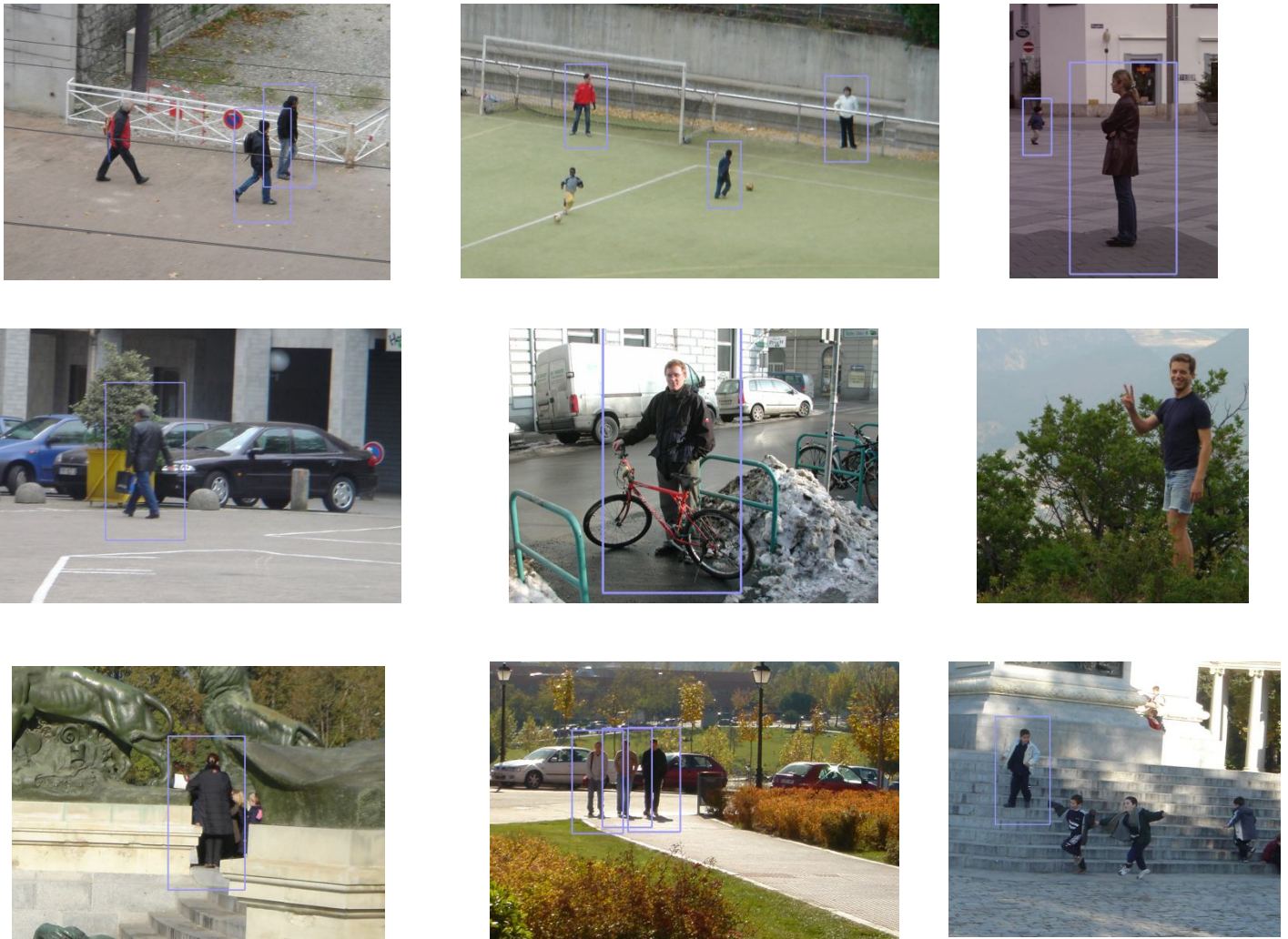
Figure 3-5: Several detection results obtained with our implementation of the Dalal-Triggs algorithm. The downscaling ratio is 1.05 and the window stride is 8 \times 8 .
